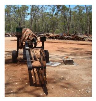
Figure 4: Buzz saw used for splitting posts
