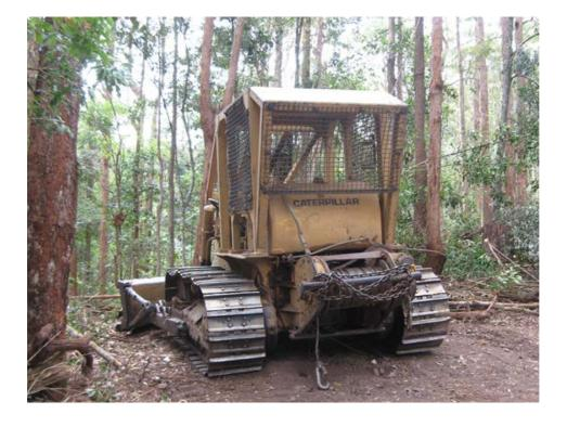
Figure 8: Dozer equipped with winch for harvesting in steep areas
