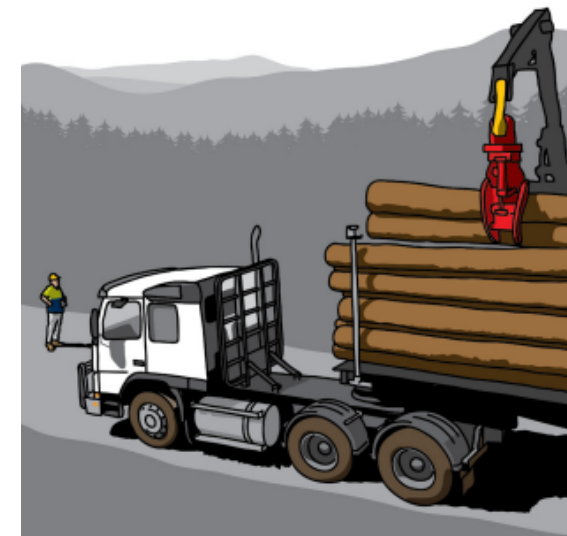
Figure 2- Example of a safe standing location a minimum of 20m from the front of the machine. Source: Guide to managing risk of loading, transporting and unloading logs
